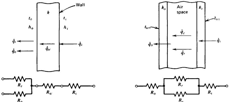
Fig. 64.12 Wall and air space illustrating thermal radiation effects.<sup>7</sup>
