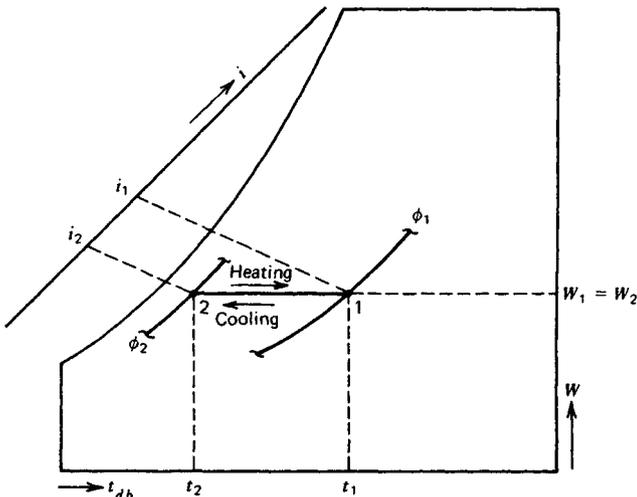
Fig. 64.3 Sensible heating and cooling process.<sup>7</sup>
