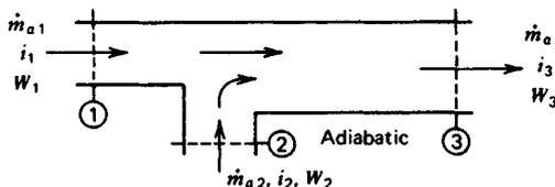
Fig. 64.9 Schematic adiabatic mixing of two air streams.<sup>7</sup>
