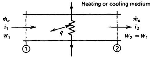
Fig. 64.2 Schematic of a heating or cooling device.<sup>7</sup>
