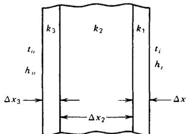
Fig. 64.13 Wall with thermal resistances in series.<sup>7</sup>
