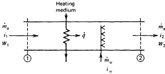
Fig. 64.6 Schematic of a heating and humidifying device.<sup>7</sup>
