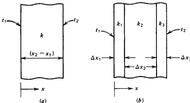
Fig. 64.11 Nomenclature for conduction in plane walls.<sup>7</sup>
