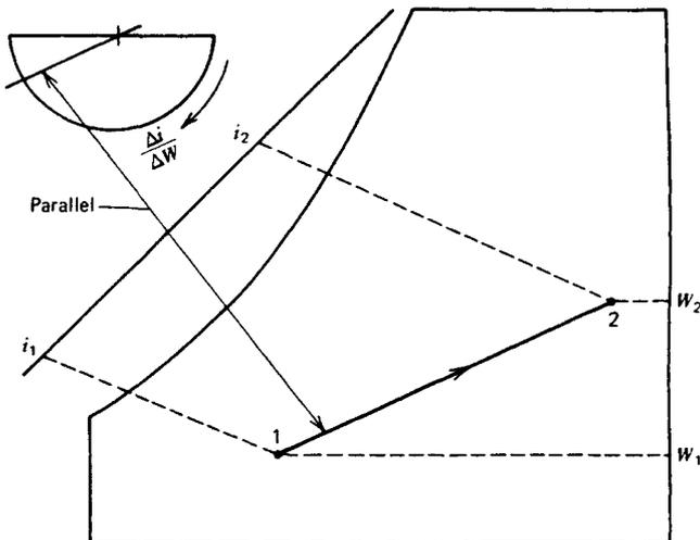
Fig. 64.7 Typical heating and humidifying process.<sup>7</sup>
