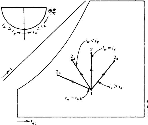
Fig. 64.8 Humidification processes without heat transfer.<sup>7</sup>
